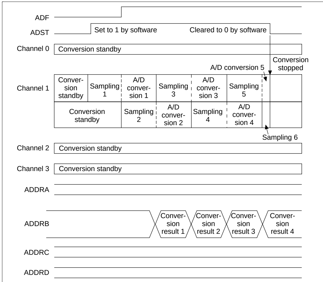
Figure 15.5 A/D Converter Operation Example (Select-Scan Mode)
