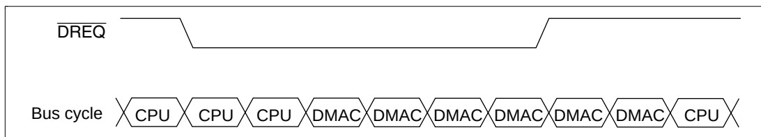
Figure 11.13 DMA Transfer Example in the Burst Mode
