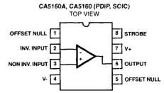
NOTE: CA5160 Series devices have an on-chip frequency compensation network. Supplementary phase-compensation or frequency roll-off (if desired) can be connected externally between terminals 1 and 8.
