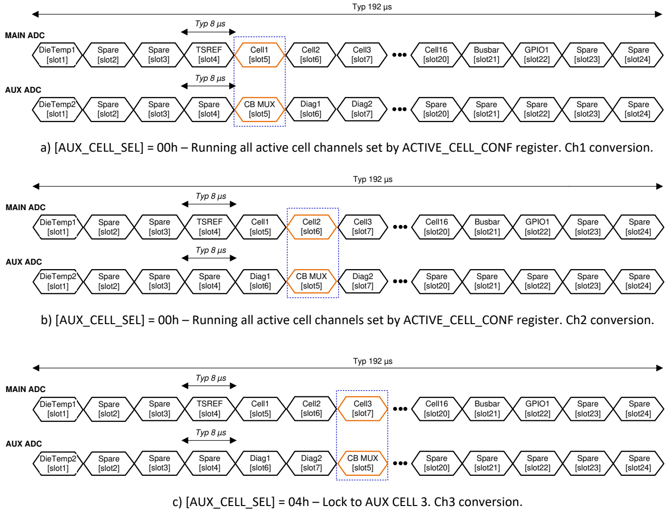
Figure 9-12. Synchronization between MAIN and AUX ADC Sampling
