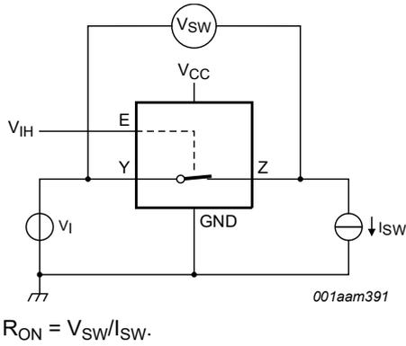
Fig. 7. Test circuit for measuring ON resistance
