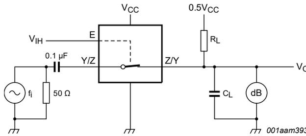
Adjust  $f_i$  voltage to obtain 0 dBm level at output. Increase  $f_i$  frequency until dB meter reads -3 dB.
