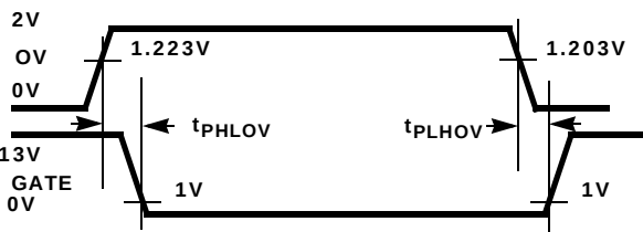
FIGURE 3A. OV TO GATE TIMING
