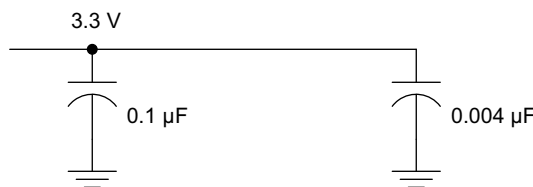
Figure 9-2. Recommended M-LVDS Bypass Capacitor Layout
