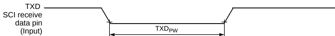
Figure 10-17 TXD Pulse Width
