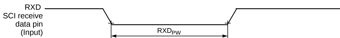
Figure 10-16 RXD Pulse Width
