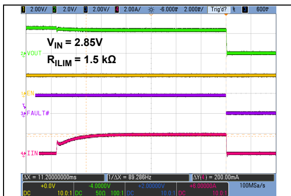
FIGURE 2-3: Overcurrent Fault Response Delay Time.
