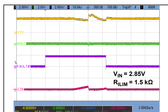
FIGURE 2-18: Turn-On into Short to GND.
