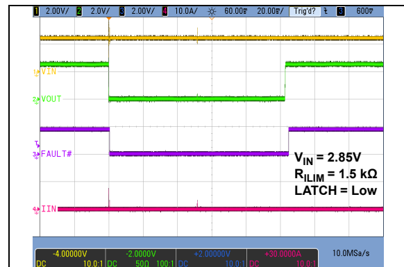
FIGURE 2-16: Output Recovery from Short Circuit.
