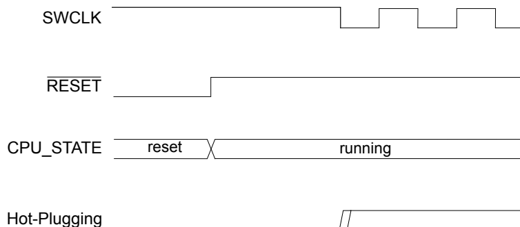
Figure 13-3. Hot-Plugging Detection Timing Diagram
