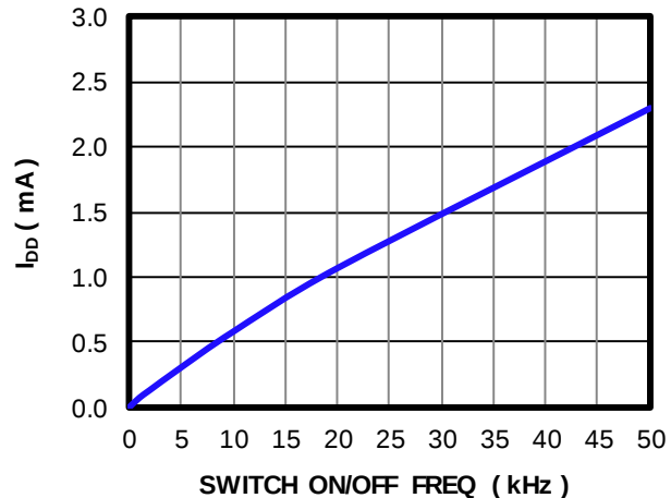
I_{DD} Vs. Switch On/Off Frequency
