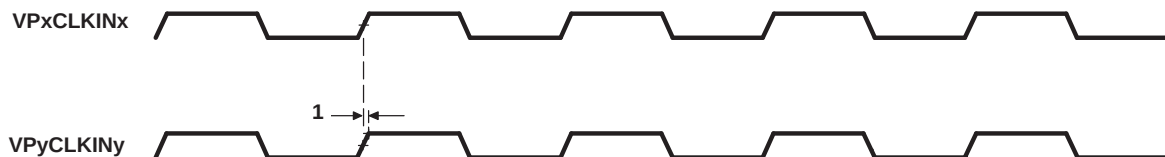
Figure 5-61. Video Port Dual-Display Sync Timing
