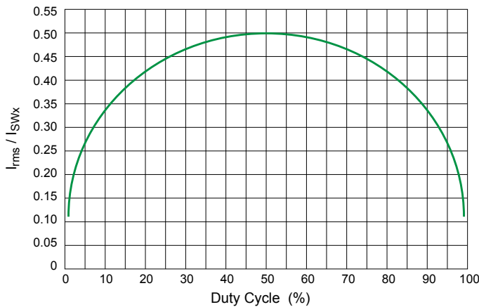
Figure 23. Input capacitor ripple versus duty cycle
