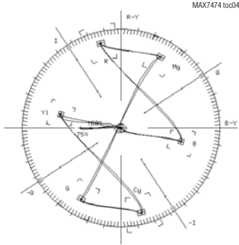
75% COLOR BAR VECTOR DIAGRAM (300m CABLE)
