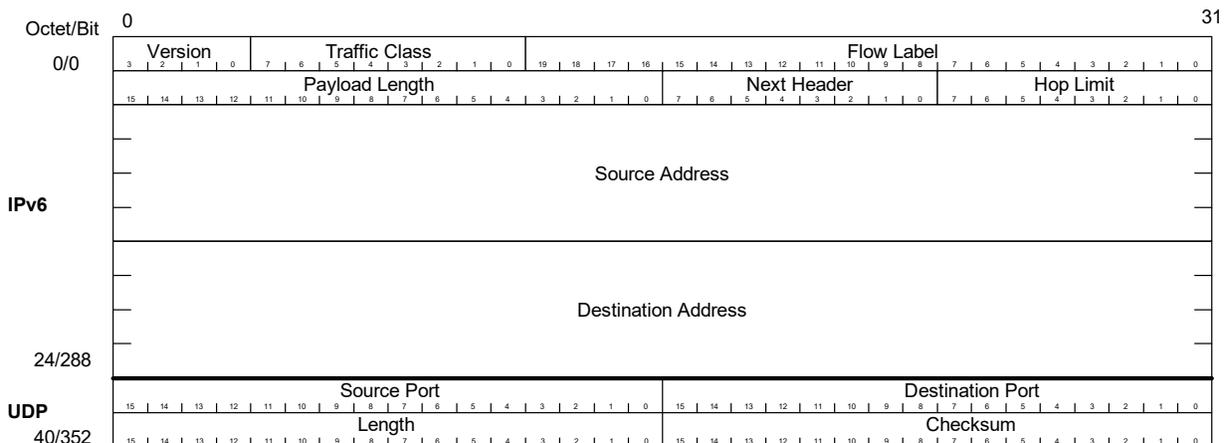
Per flow validation is performed on the Source or Destination Address in the IPv6 header. The comparator can be configured to indicate a match in the flow if the source, destination, or either the source or destination fields match.
