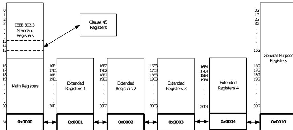
**Reserved Registers** For main registers 16–31, extended registers 16E1–30E1, 16E2–30E2, 16E3–30E3, 16E4–30E4, and general purpose registers 0G–30G, any bits marked as Reserved should be processed as read-only and their states as undefined.
