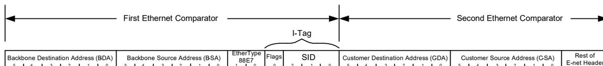
**Figure 79 • PBB Ethernet Frame Format (1 B-Tag)**
