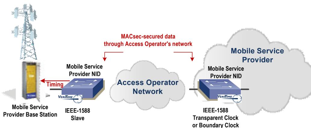
The mobile service provider may choose to leave VLAN tags or MPLS labels unencrypted so that the access operator can map the virtual private line services.
