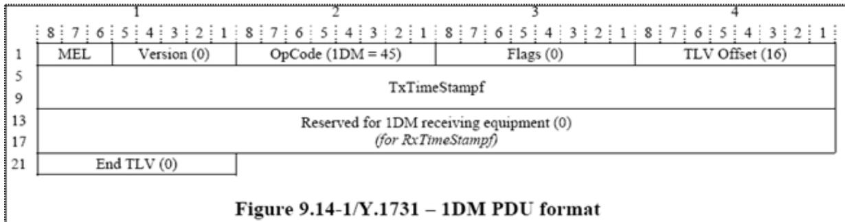
1. For one-way delay measurements, both MEPs must support IEEE 1588 and be in sync.
