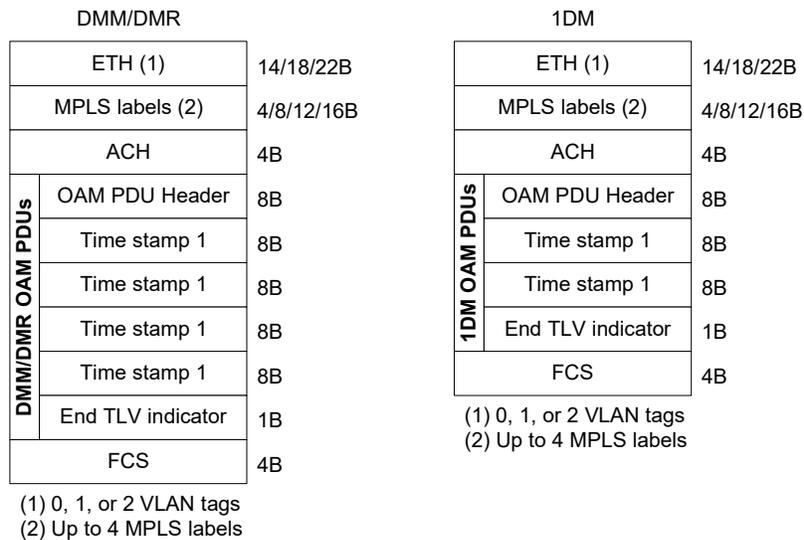
As with PTP, there is no protocol validation for MPLS OAM; only interpretation of the header to determine what action to take. The first four bytes of the header are used to determine the action to be taken.
