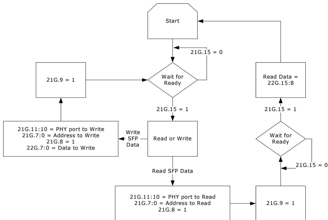
To read a value from a specific address of the two-wire serial slave device:
