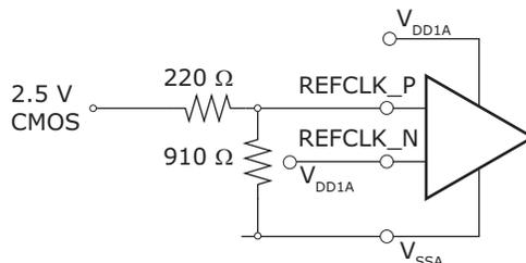
**Figure 49 • 3.3 V CMOS Single-Ended REFCLK Input Resistor Network**
