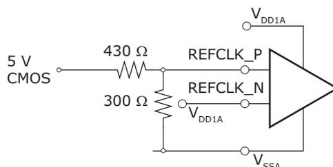
**Note:** A single-ended 25 MHz reference clock is not guaranteed to meet requirements for QSGMII MAC operation.
