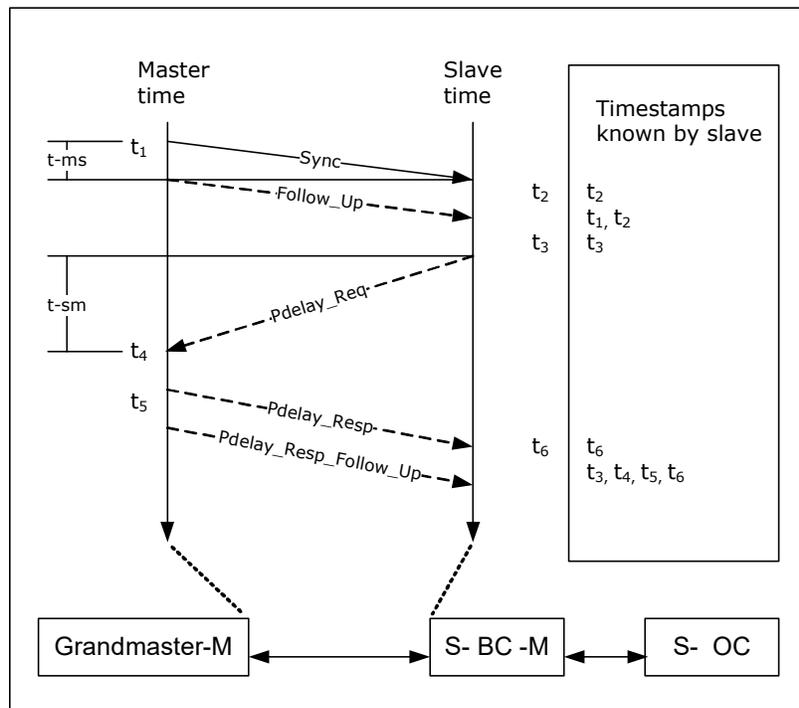
To calculate the path delays on a link, the IEEE 1588 engine (located somewhere in the system) generates Pdelay\_req messages on all ports. When transmitted, the actual Tx time stamp  $t_3$  is saved for the CPU to read.
