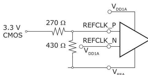
**Figure 50 • 5 V CMOS Single-Ended REFCLK Input Resistor Network**
