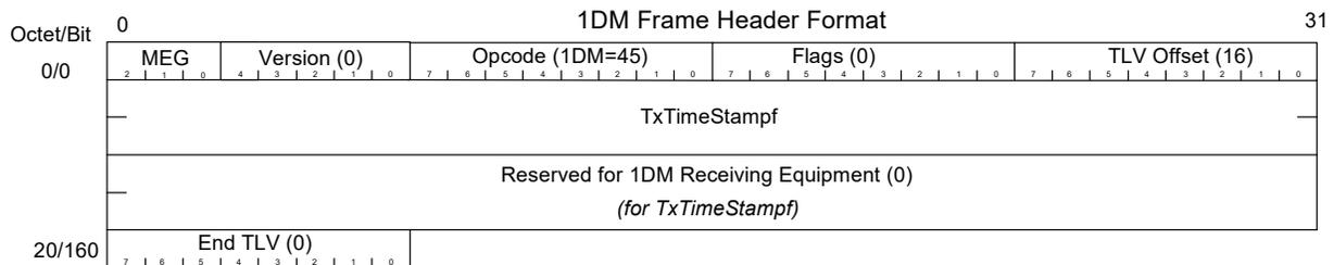
The following illustration shows a DMM frame header.
