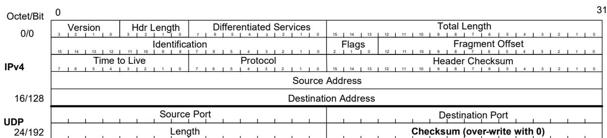
**Note:** Checksum over-write with 0 occurs on ingress only. PTP applications that generate 1588 frames with this format are responsible for creating IPv4/UDP frames with a zeroed checksum upon generation from the application.
