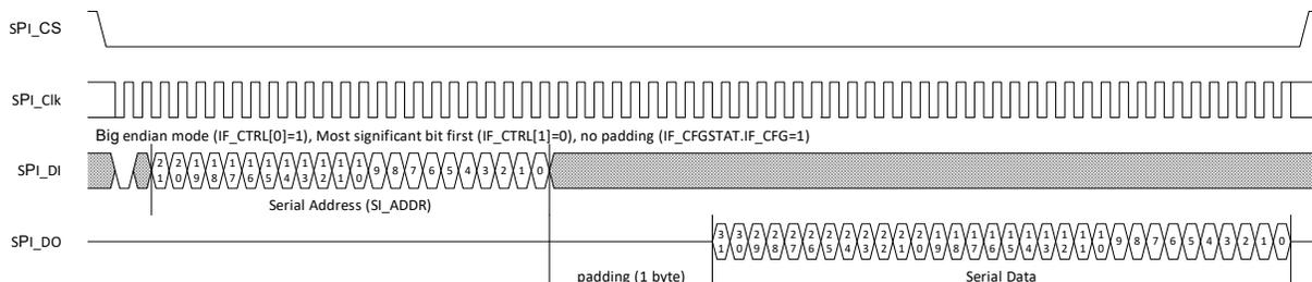
A 25 MHz SPI operating rate is used to access the CSR address space.
