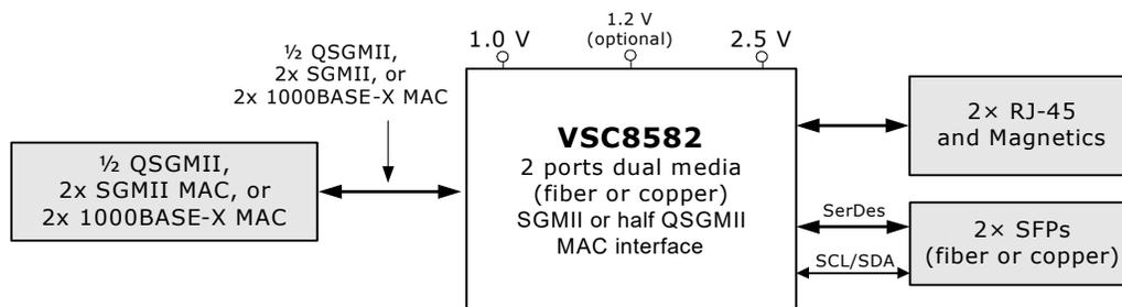
**Figure 2 • Copper Transceiver Application Diagram**
