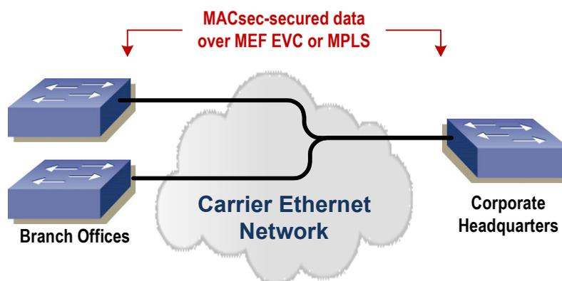
With traditional MACsec, VLAN tags or MPLS labels are fully encrypted and hidden from the Carrier Ethernet network thereby limiting the enterprise to only the simplest point-to-point private line connectivity services.
