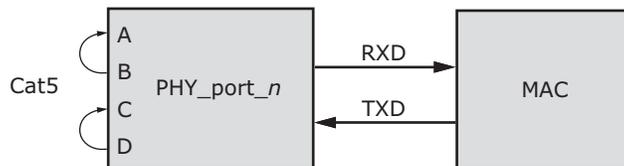
When using the connector loopback testing feature, the device autonegotiation, speed, and duplex configuration is set using device registers 0, 4, and 9. For 1000BASE-T connector loopback, the following additional writes are required. Execute the additional writes in the following order:
