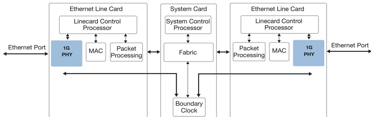
This solution also works for pizza boxes. To ensure that blade redundancy works, if the PHYs for the redundant blades must have the same 1588-in-the-PHY configuration.
