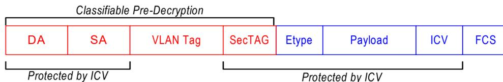
**Figure 31 • Dual-Tagged Ethernet**
