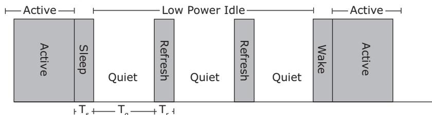
Using LPI, the usage model for the link is to transmit data as fast as possible and then return to a low power idle state. Energy is saved on the link by cycling between active and low power idle states. During LPI, power is reduced by turning off unused circuits and using this method, energy use scales with bandwidth utilization.
