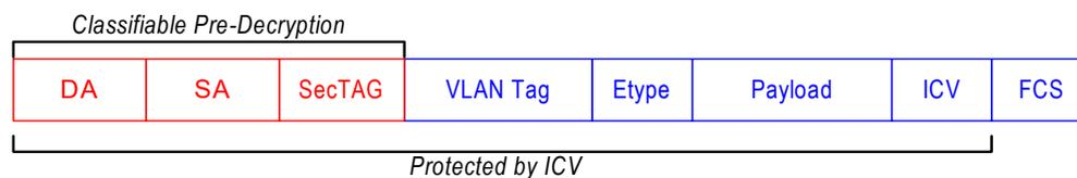
**Figure 27 • Dual-Tagged Ethernet**
