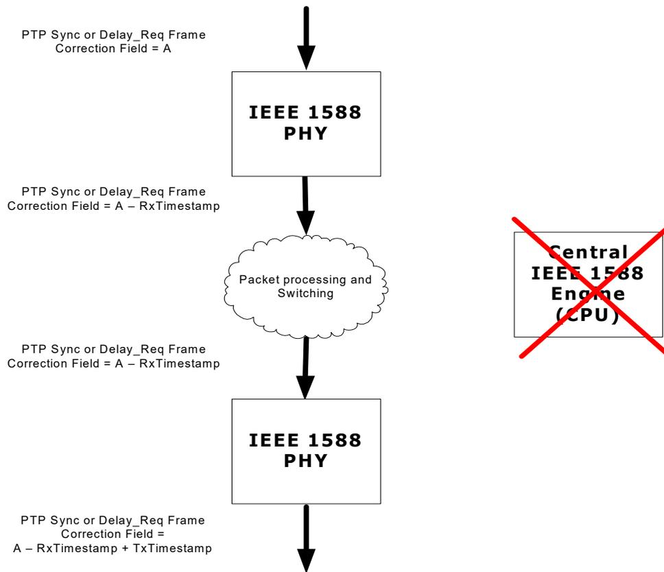
When the system works in one-step E2E TC mode Sync and Delay\_req frames must be forwarded through the system and the residence time = (Egress time stamp – Ingress time stamp) must be added to the correction field in the frame before it leaves the system.
