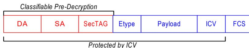
**Figure 25 • Single-Tagged Ethernet**
