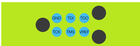
Figure 51: Foot print for tag-connect header
