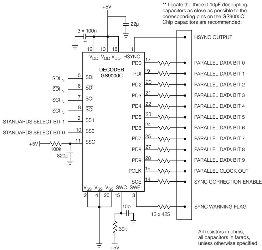
With synchronized serial data and clock connected to the GS9000C, the HSYNC output (pin 1) will toggle for each HSYNC detected. The Parallel Data bits PD0 through PD9 and the Parallel Clock can be observed on an oscilloscope or fed to a logic analyzer. To directly drive parallel inputs to receiving equipment, such as monitors or digital to analog converters, these outputs can be fed through a suitable TTL to ECL converter.
