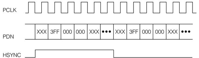
Fig. 10 Operation of HSYNC with Respect to PCLK
