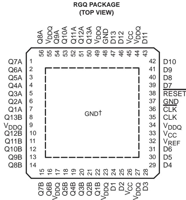
† The center die pad must be connected to GND.
