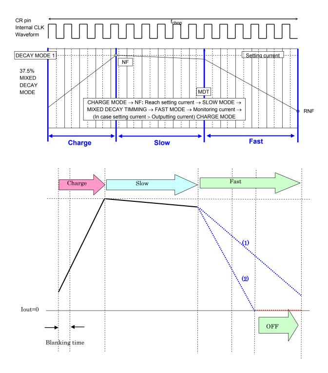
The [NF] shows the point where the output current reaches the setting current value. The [Charge] shows the different value depending on the step resolution characteristics (inductance or resistance).
