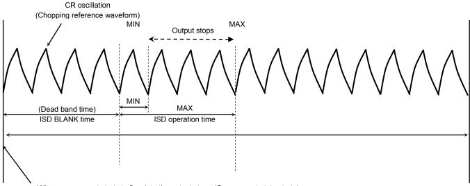
When over-current starts to flow into the output stage (Over-current state starts)
