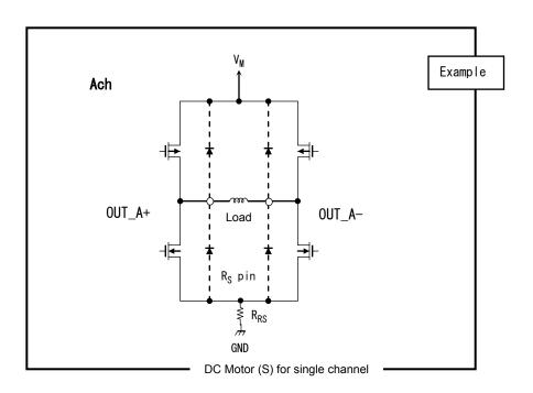
o ...Indicates an IC output pin connected to a motor.
