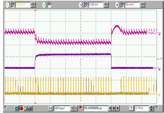
Top: Vo2, CH2 Output Voltage Ripple, (50mV/div) Middle: Io2, CH2 Output Current, (5A/div) Bottom: SWN2, CH2 Switching Node Voltage, (10V/div) Time: 20μs/div
