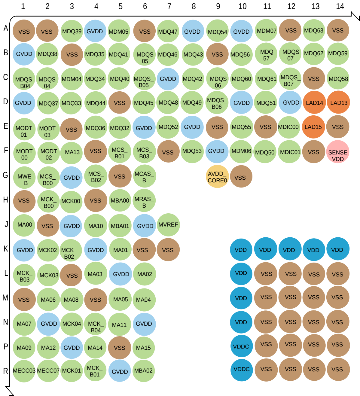
Figure 3. P1022 detail A ball map
