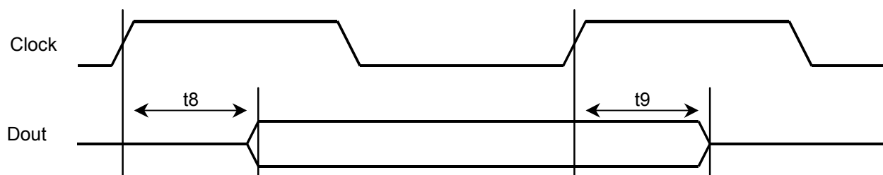
Figure 18-5. To/From High-Z Delay Definitions (Rising Clock Edge)
