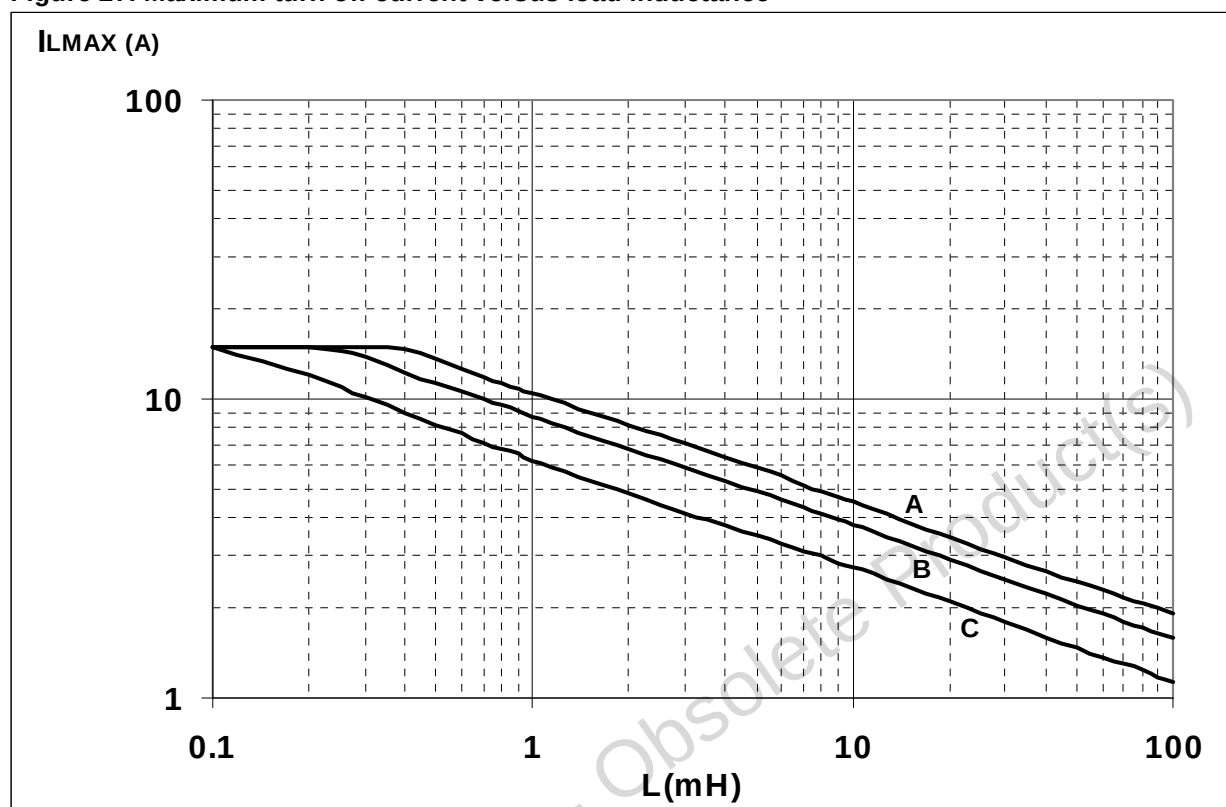
Figure 27. Maximum turn off current versus load inductance
