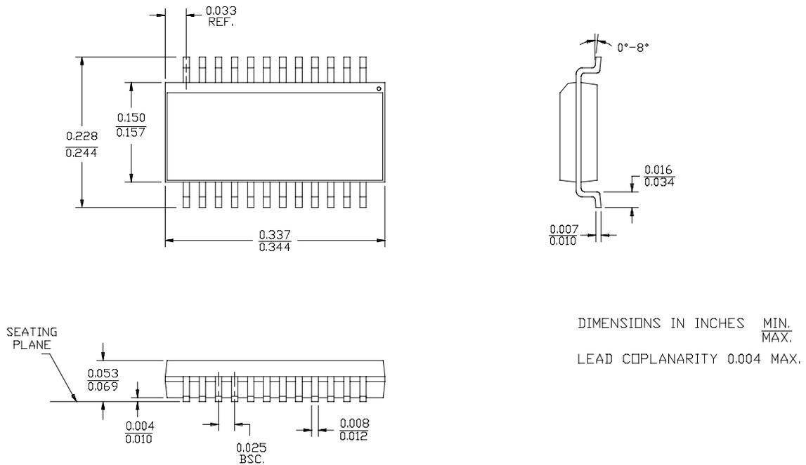
**24-Lead (300-Mil) Molded SOIC S13**
