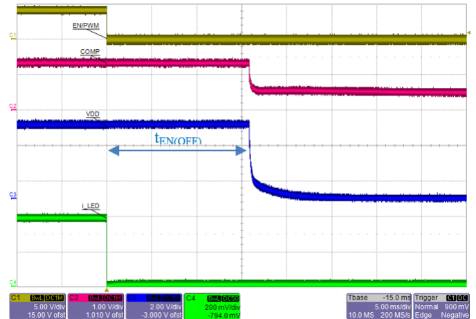
Figure 29: After EN/PWM (Yellow) goes Low for ~16 ms, the IC completely shuts down so both VDD (Blue) and COMP (Red) decay.
