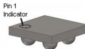
Figure 4. WLCSP Bumps Facing Down (Bottom View)
