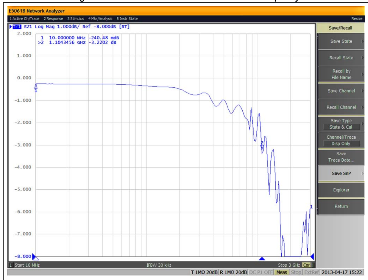
Figure 22. Data switch transfer characteristics vs. frequency
