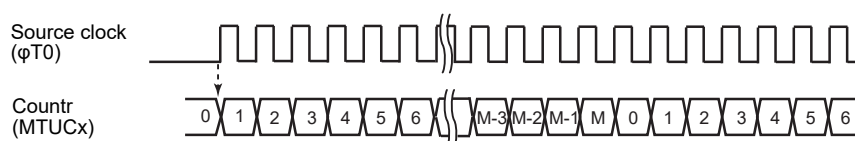
Figure 24-4 Count-up/clear operation when \phi T0 is selected as a source clock
