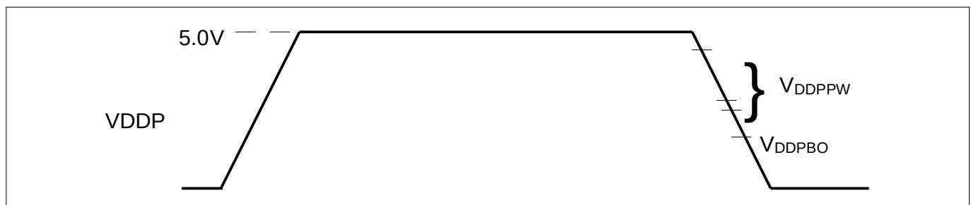
Figure 14 Supply Threshold Parameters
