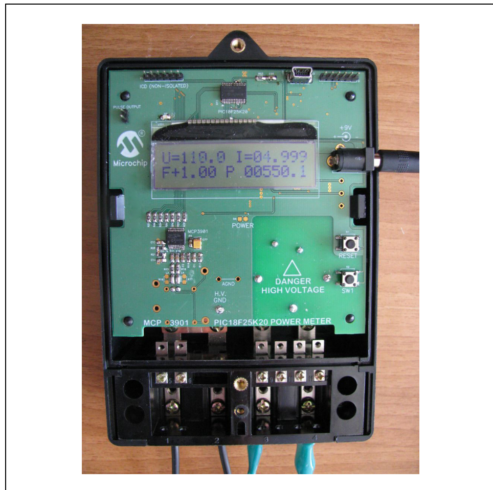
FIGURE 1-1: MCP3901 Low-Cost Power Monitor Reference Design
