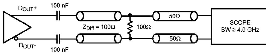
FIGURE 6. Serializer CML Output Load and Transition Times
