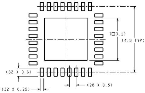
DIMENSIONS ARE IN MILLIMETERS
