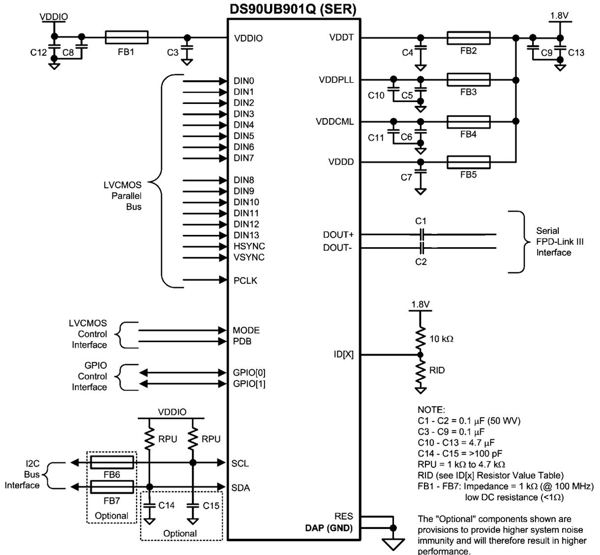
FIGURE 37. DS90UB901Q Typical Connection Diagram — Pin Control
