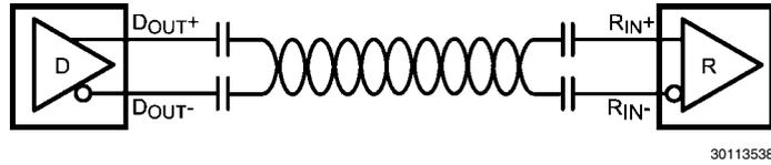
FIGURE 36. AC-Coupled Connection
