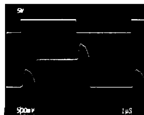
MUX-08 SMALL-SIGNAL SWITCHING
