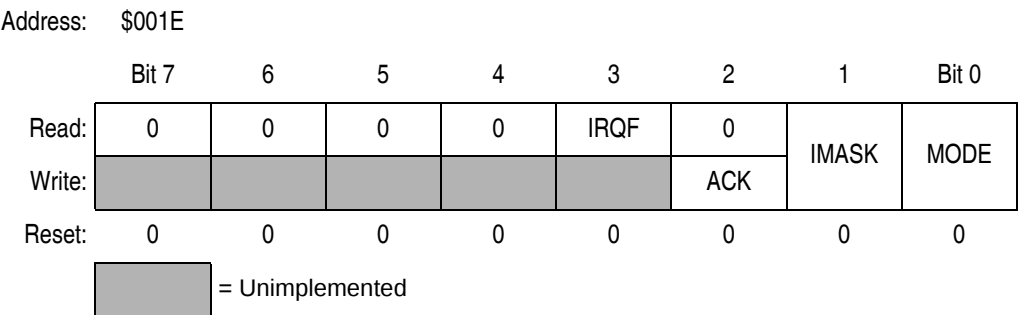
Figure 15-3. IRQ Status and Control Register (ISCR)
