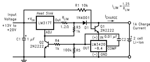
**Figure 14. Constant Current/Constant Voltage Li-Ion Battery Charger**
