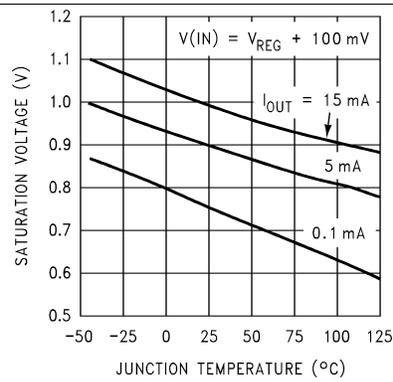
**Figure 7. Output Saturation Voltage ( $V_{SAT}$ )**
