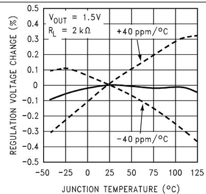
Figure 6. Normalized Temperature Drift
