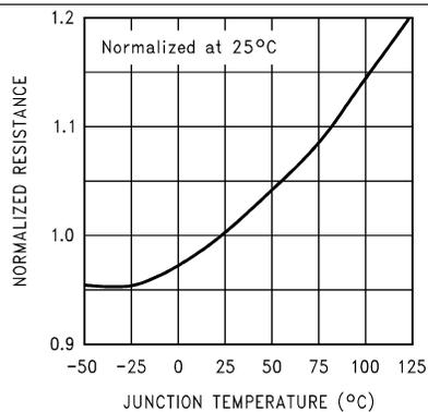
Figure 5. Internal Feedback Resistor ( $R_f$ ) Tempco
