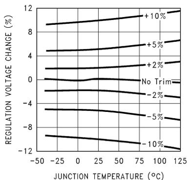
Figure 11. Normalized Temperature Drift With Output Externally Trimmed
