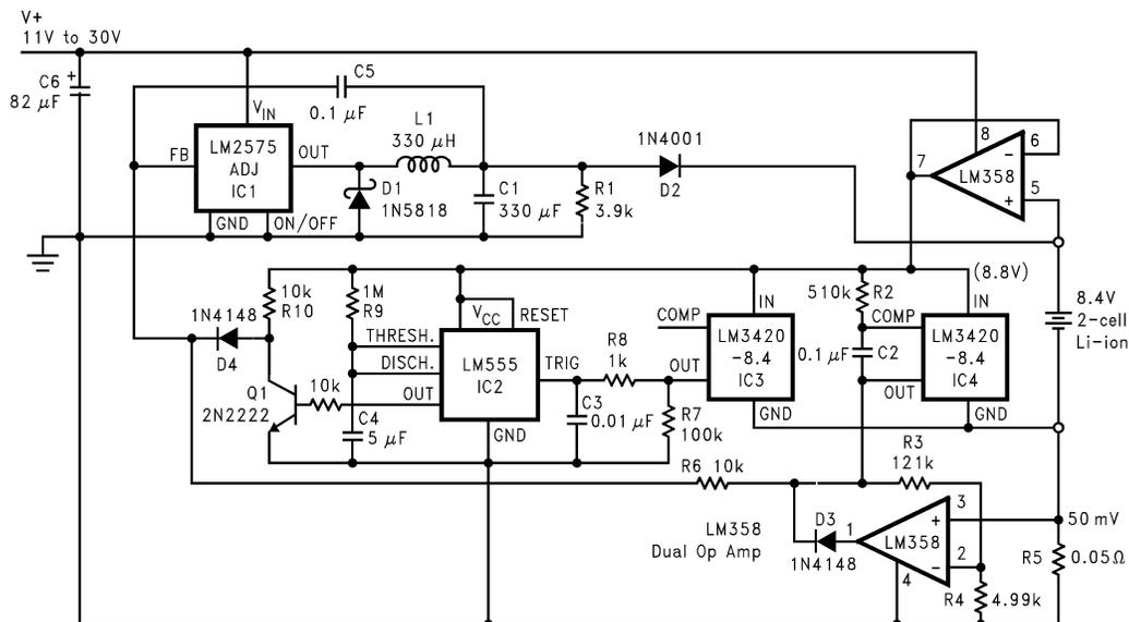
Figure 20. (Fast) Pulsed Constant Current 2-Cell Charger
