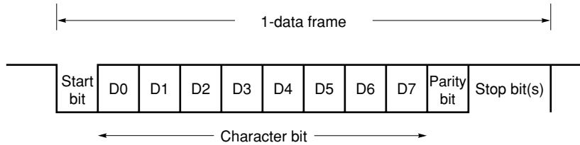
Figure 17-7. Asynchronous Serial Interface Transmit/Receive Data Format
