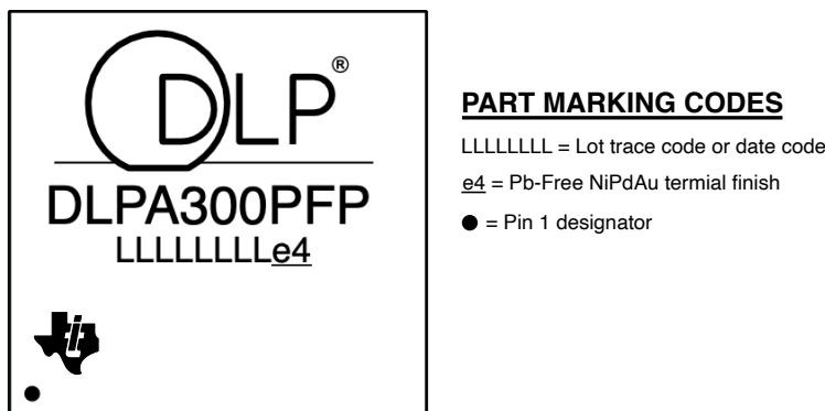
Figure 11-1. Device Marking (Device Top View)
