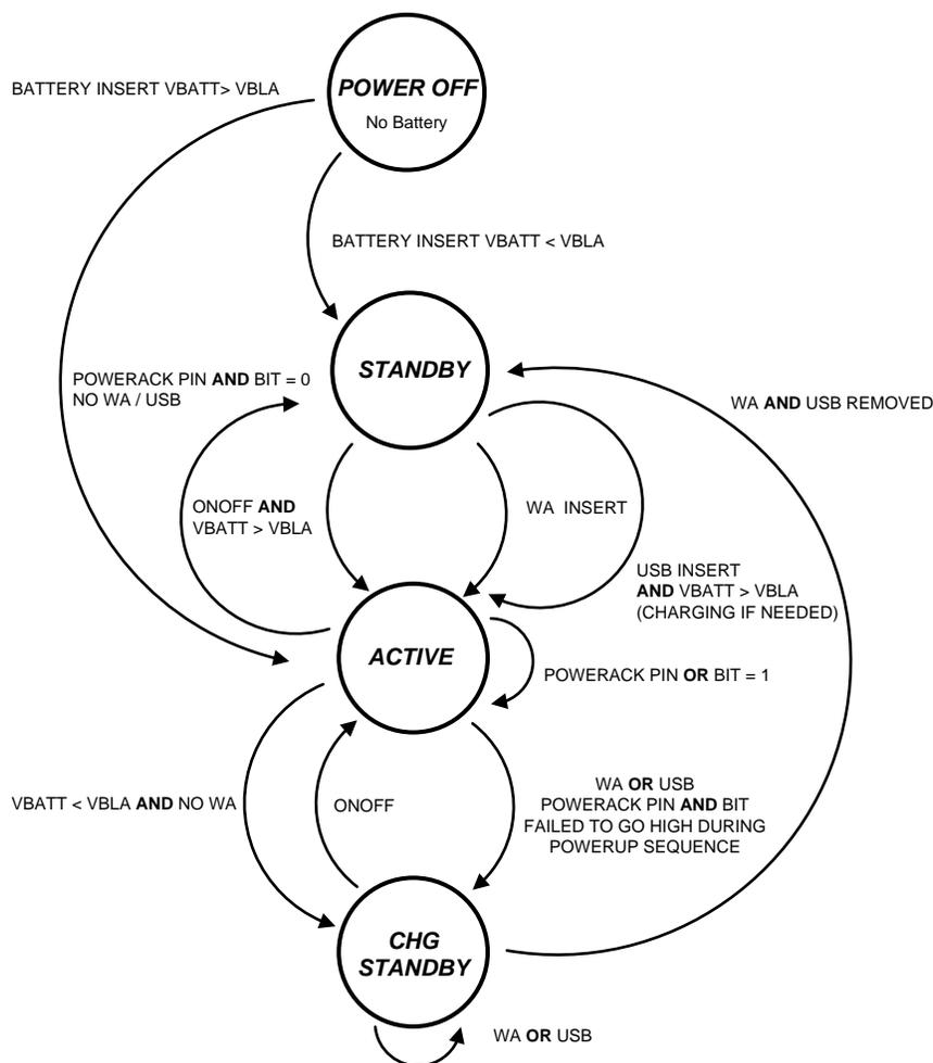
Figure 53. Operating Mode State Diagram
