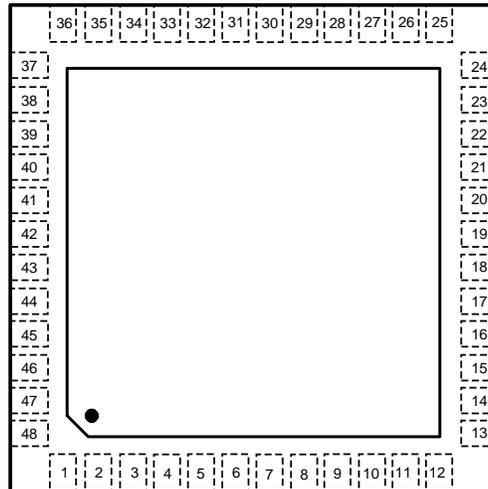
**Figure 1. 48 WQFN Package (Top View)
