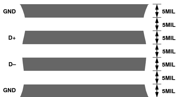
Figure 34. Typical Arrangement of Signal Tracks
