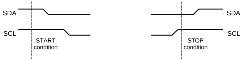
Figure 13-3. START and STOP Conditions
