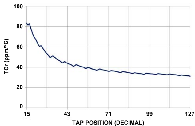
FIGURE 16. 50kΩ TCr vs TAP POSITION, V_{CC} = 3.3V
