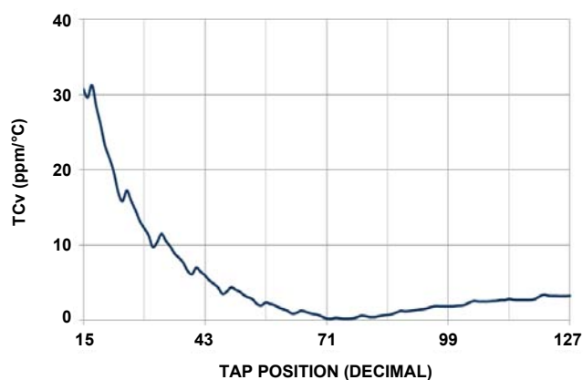
FIGURE 14. 50kΩ TCv vs TAP POSITION, V_{CC} = 3.3V
