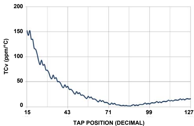
FIGURE 13. 10kΩ TCv vs TAP POSITION, V_{CC} = 3.3V
