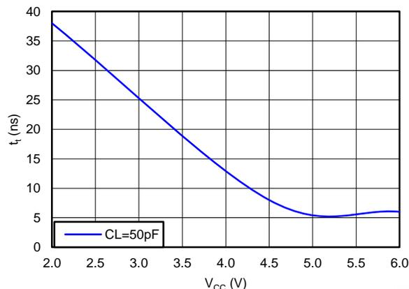
Figure 4. Transition Time vs  $V_{CC}$
