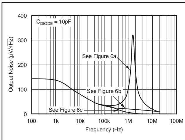
Figure 8. Output Noise for Circuits in Figure 6
