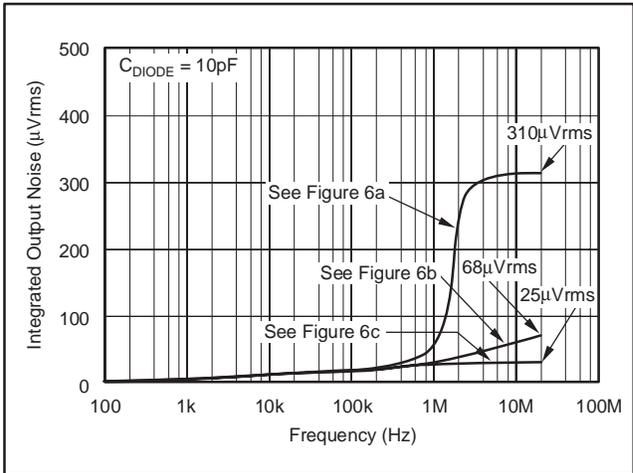
Figure 9. Integrated Output Noise for Circuits in Figure 6
