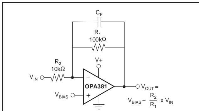
**Figure 14. Inverting Gain**
