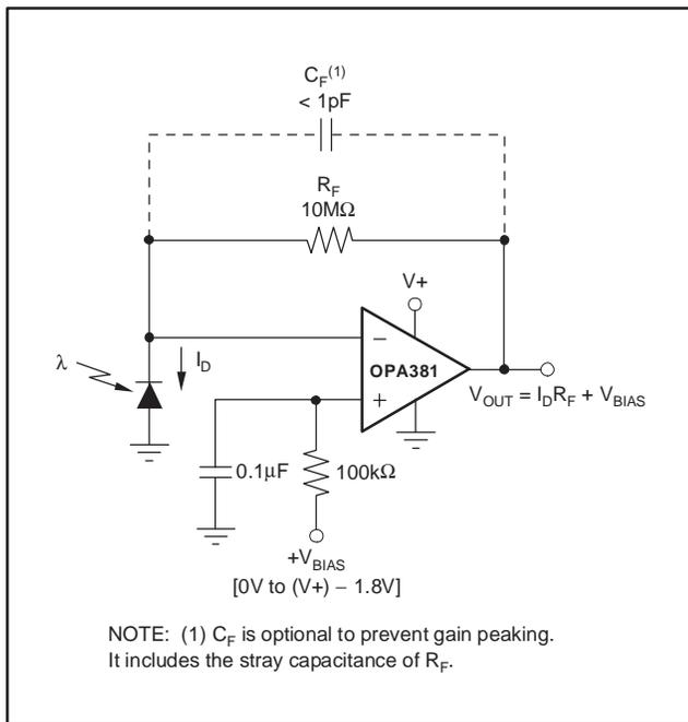
**Figure 4. Photodiode with Filtered Reverse Bias Voltage**
