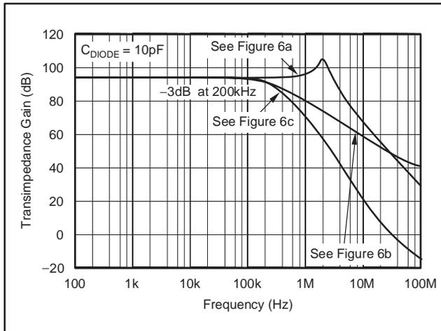
Figure 7. Transimpedance Gains for Circuits in Figure 6
