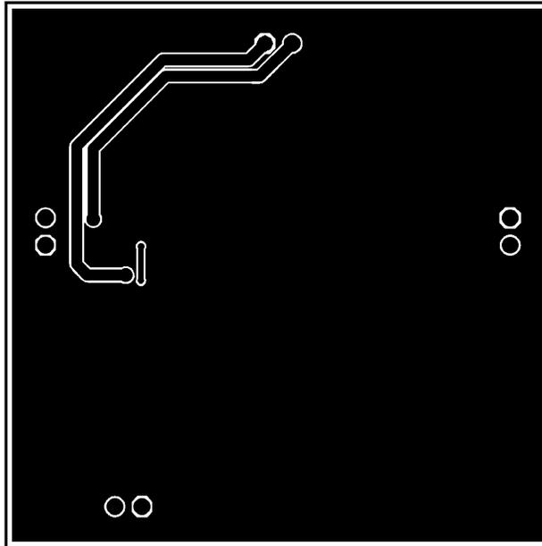
Figure 24. Recommended SD PCB Layout
