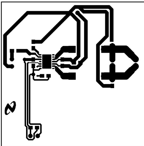
Figure 23. Recommended SD PCB Layout
