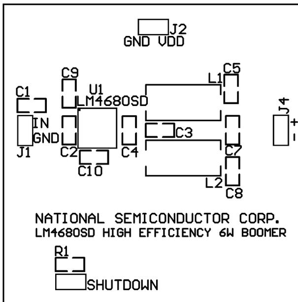
Figure 22. Recommended SD PCB Layout
