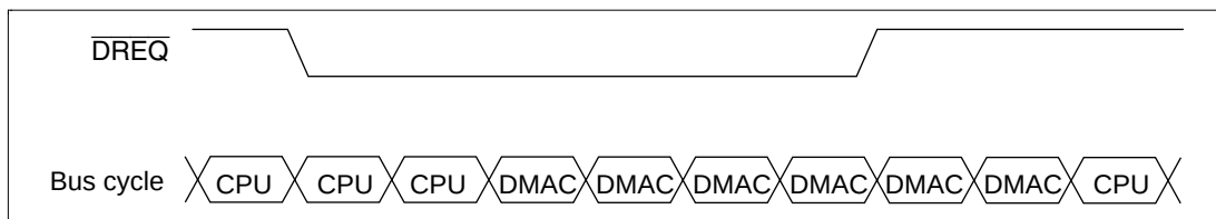
Figure 11.13 DMA Transfer Example in the Burst Mode
