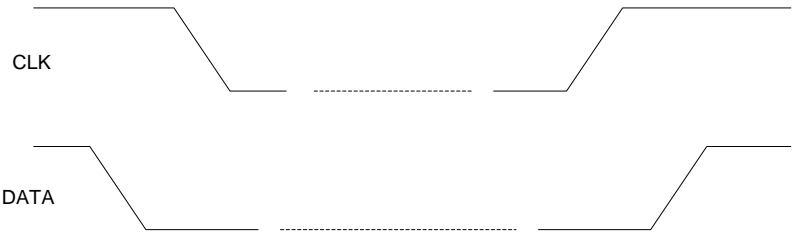
Figure 18: Timing of START and STOP Condition
