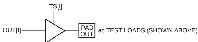
Figure 74. ac Test Loads
