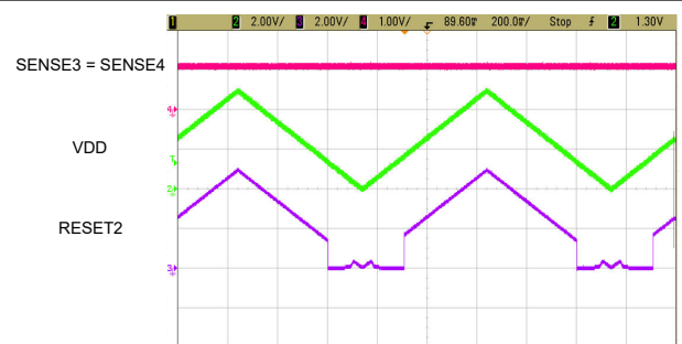
Figure 9-8. TPS37044-Q1 Overvoltage and Undervoltage Function
