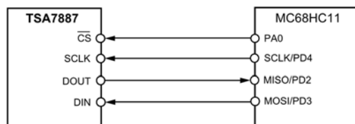
Figure 18: Interfacing the TSA7887 to 68HC11-type Microcontrollers.
