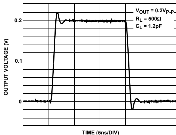
FIGURE 14. SMALL SIGNAL TRANSIENT RESPONSE; R_L = 500\Omega
