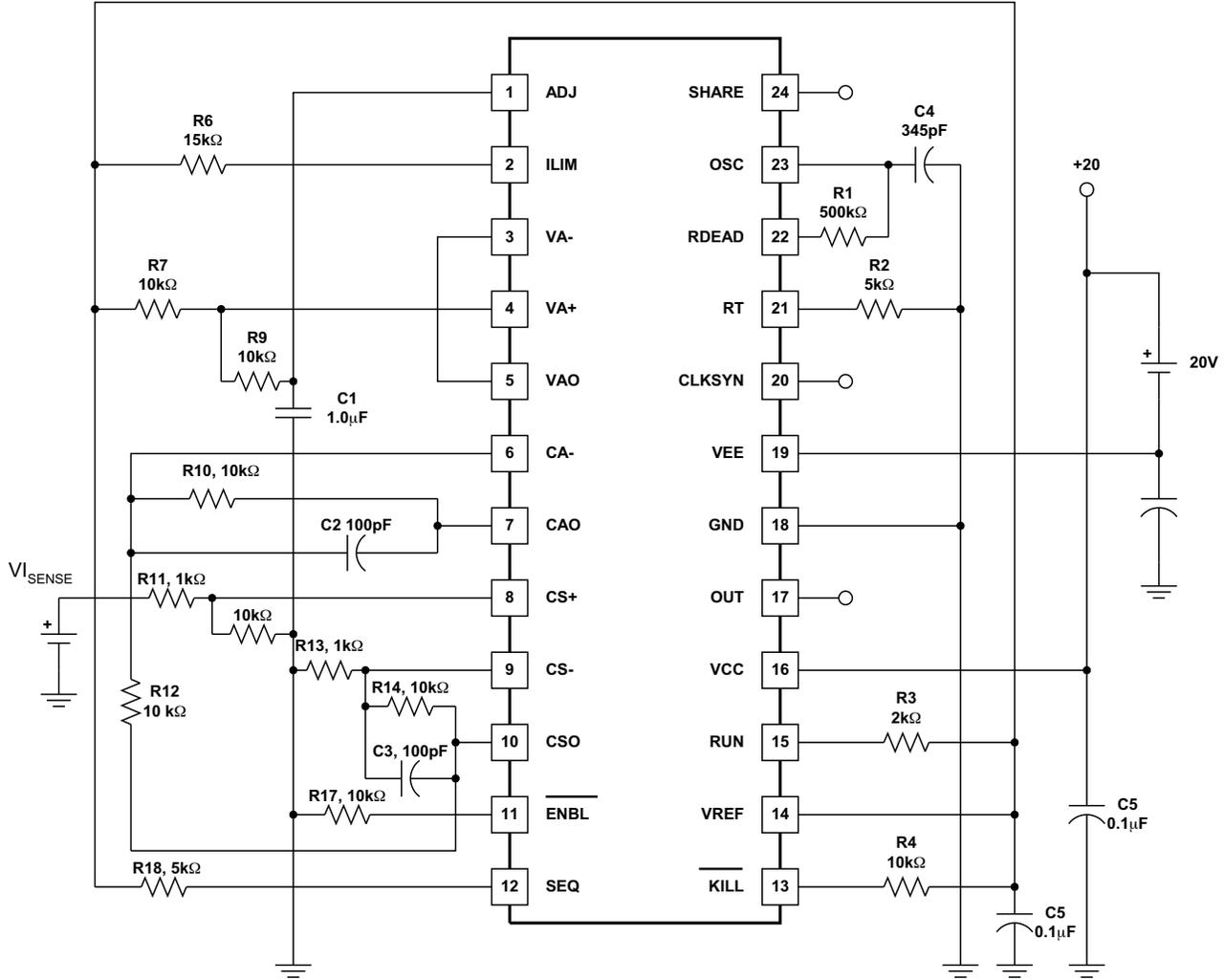
Figure 9. Open Loop Circuit
