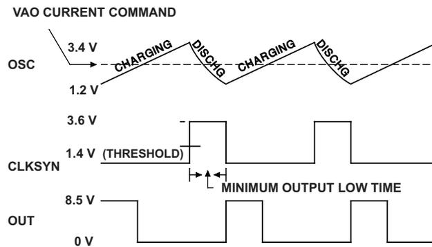
**Figure 2. Oscillator and PWM Output Waveform**
