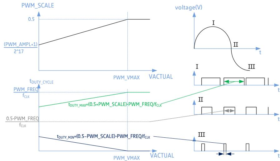
Figure 57: Calculation of PWM Duty Cycles ( $PWM\_AMPL$ )
