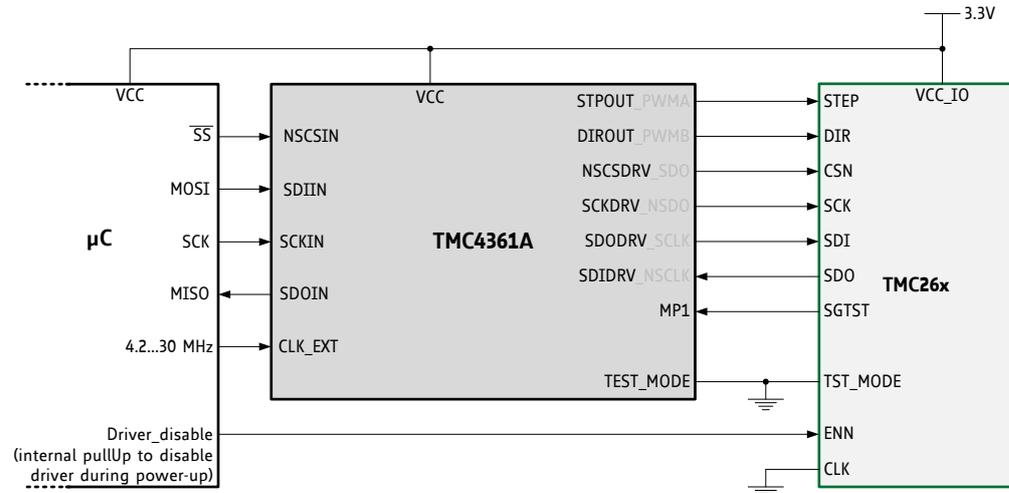
Figure 81: TMC4361A with TMC26x Driver in SPI Mode
