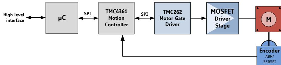
Figure 4: Hardware Set-up for Closed-loop Operation with TMC262
