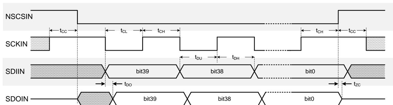
Figure 14: SPI Timing Datagram
