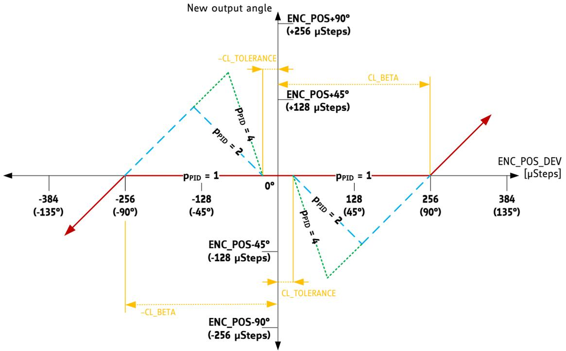
Figure 66: Calculation of the Output Angle with appropriate CL\_DELTA\_P
