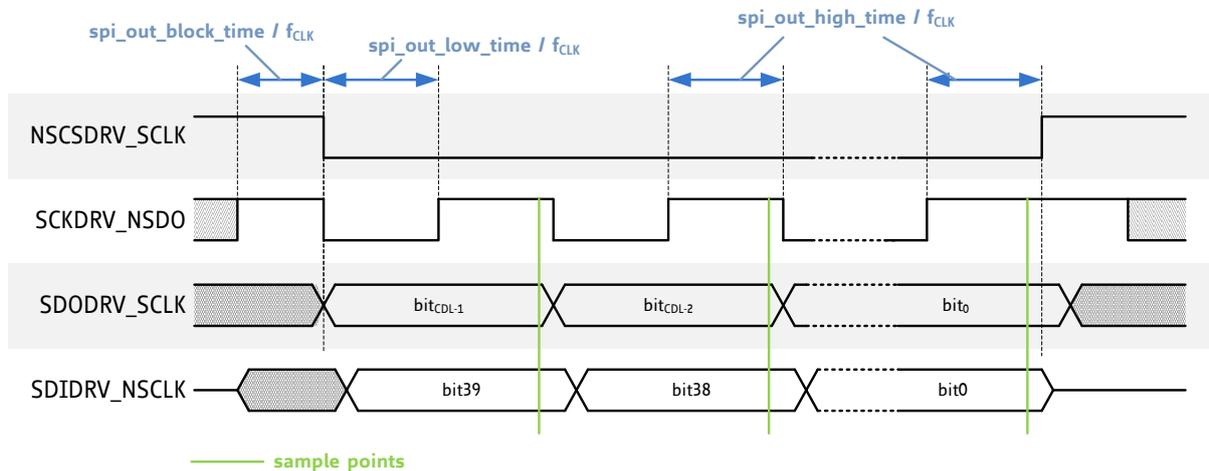
Figure 53: SPI Output Datagram Timing
