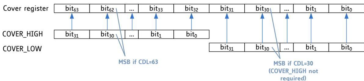
Figure 54: Cover Data Register Composition (CDL – `COVER_DATA_LENGTH`)
