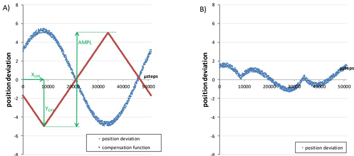
Figure 61: Triangular Function that compensates Encoder Misalignments
