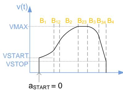
*Using  $VSTART$  and starting acceleration, which is smaller than  $AMAX$  for S-shaped ramps*
