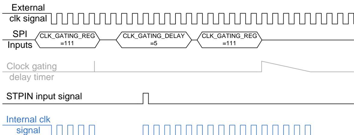
Figure 70: Manual Clock Gating Activation and Wake-Up
