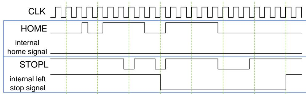
Figure 15: Reference Input Pins:  $SR\_REF = 1$ ,  $FILT\_L\_REF = 1$
