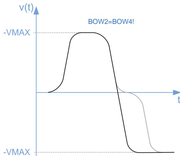
Figure 32: Direct transition via  $V_{ACTUAL}=0$  for S-shaped Ramps
