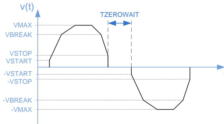
Figure 30: Example for U-Turn Behavior of sixPoint Ramp
