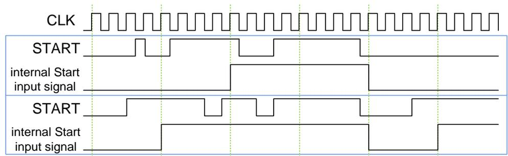
Figure 16: START Input Pin:  $SR\_S = 2$ ,  $FILT\_L\_S = 0$
