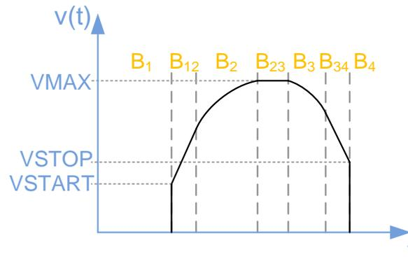
Figure 27: S-shaped Ramp with Start and Stop Velocity
