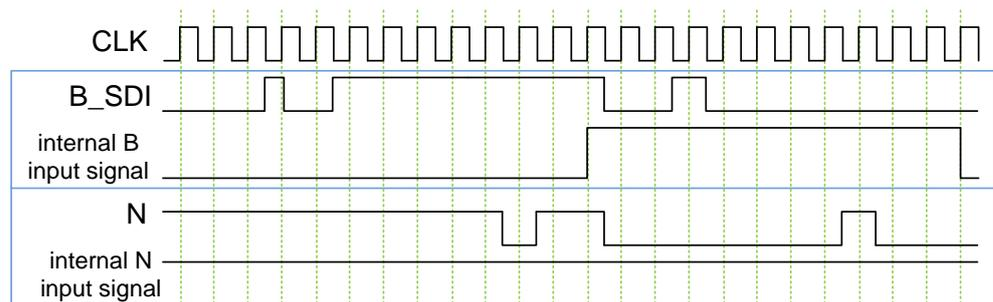
Figure 17: Encoder Interface Input Pins:  $SR\_ENC\_IN = 0$ ,  $FILT\_L\_ENC\_IN = 7$
