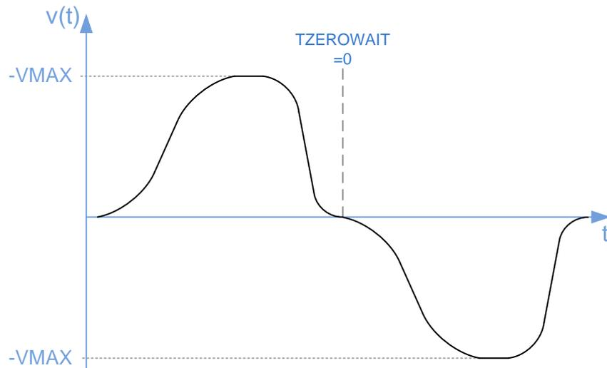
Figure 31: Example for U-Turn Behavior of S-shaped Ramp
