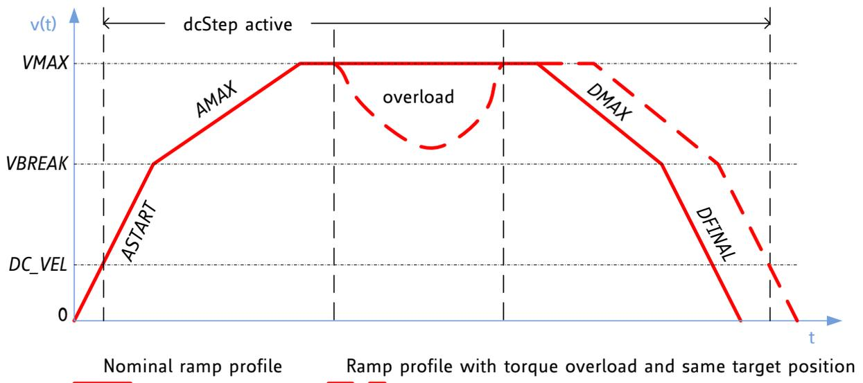
Figure 60: Velocity Profile with Impact through Overload Situation
