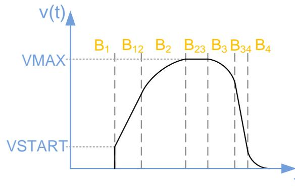
Figure 25: S-shaped Ramp with initial Start Velocity
