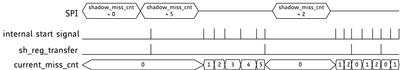
Figure 41: *SHADOW\_MISS\_CNT* Parameter for several internal Start Signals
