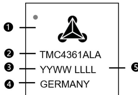
Figure 79: Marking Details on Chip<sup>1</sup>
