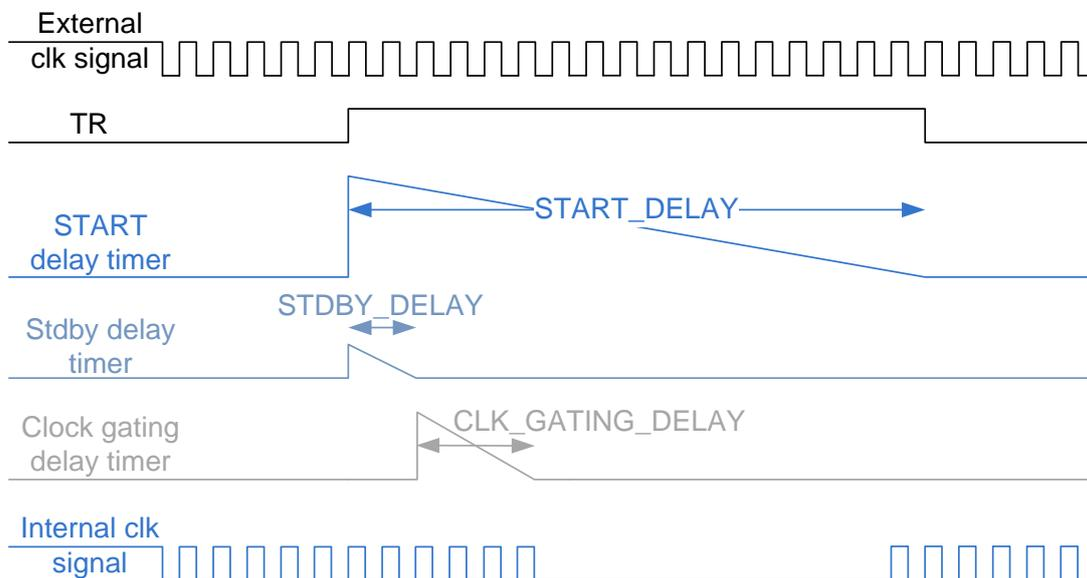
Figure 71: Automatic Clock Gating Activation and Wake-Up
