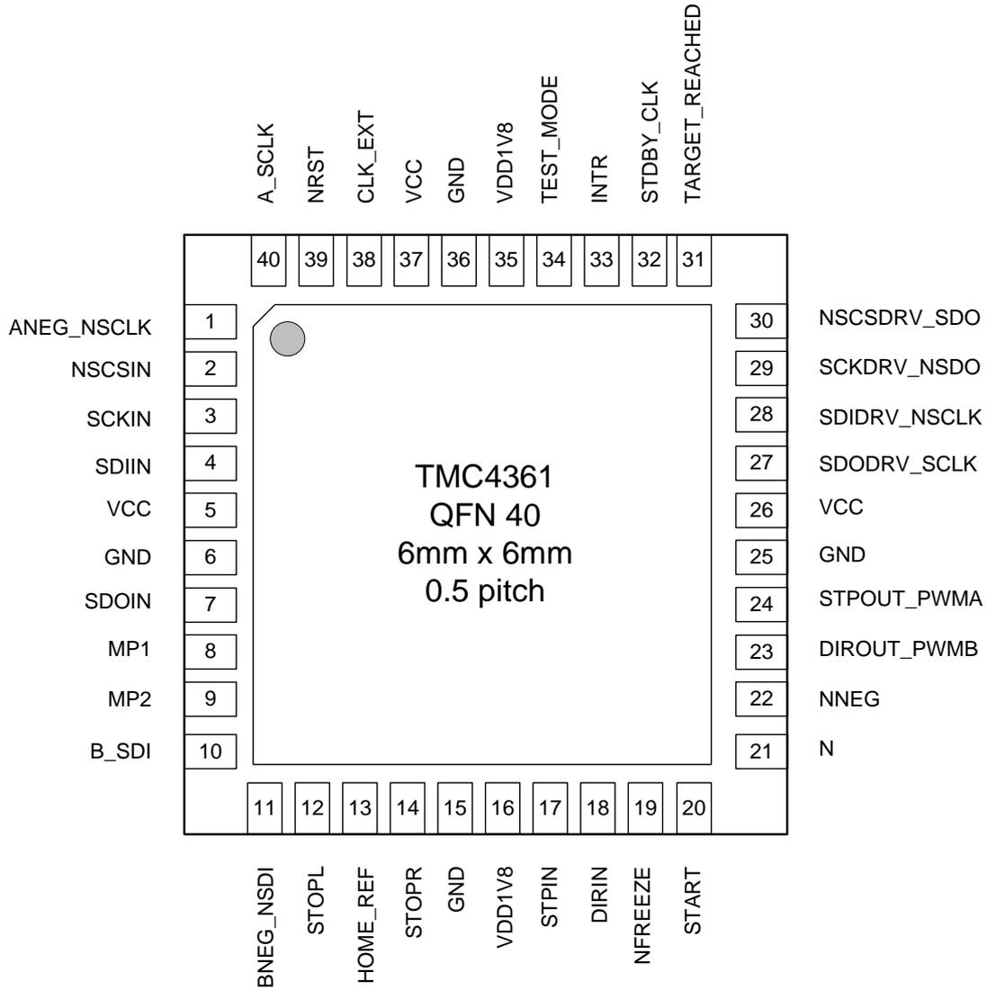
Figure 6: Package Outline: Pin Assignments Top View
